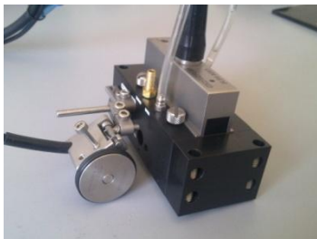
Phased Array linear UT probe with wedge made of Aqualenne
